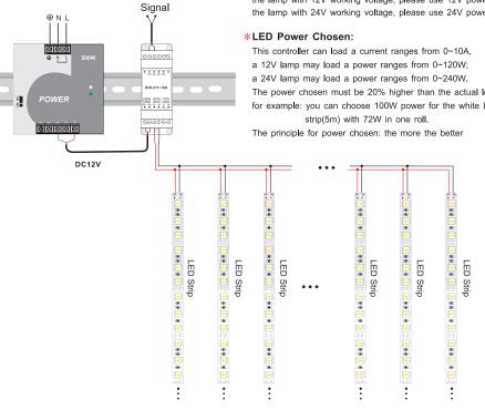
2) Connection Diagram for Multiple Units:
